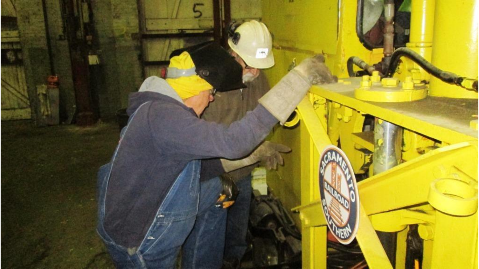
Cliff and Alan work on a new locking-latch for the tie-shear's kickers
