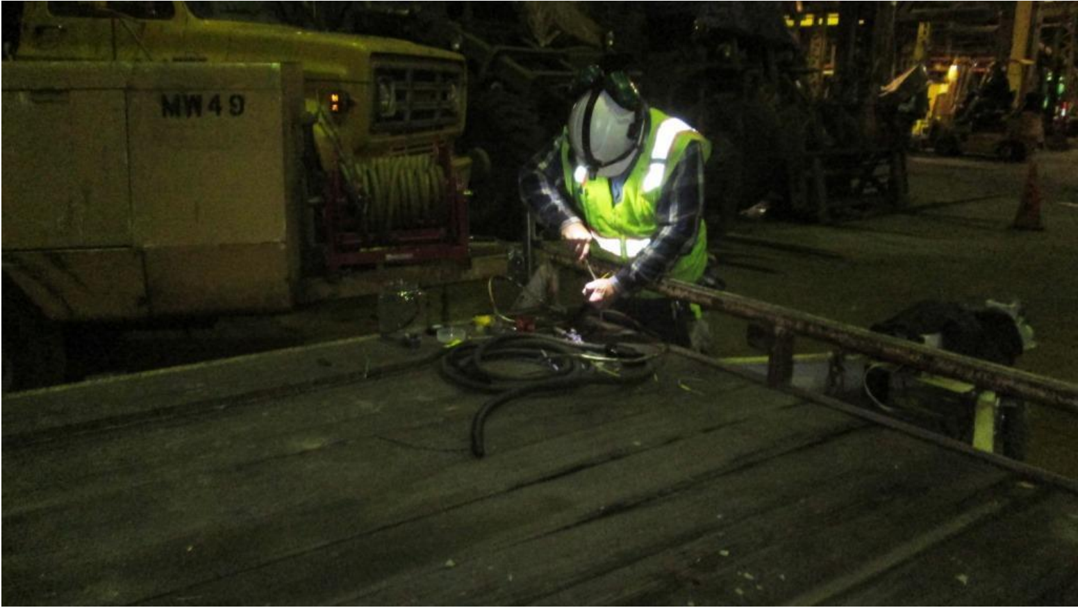
Joe repairs the hitch-wires on the trailer
