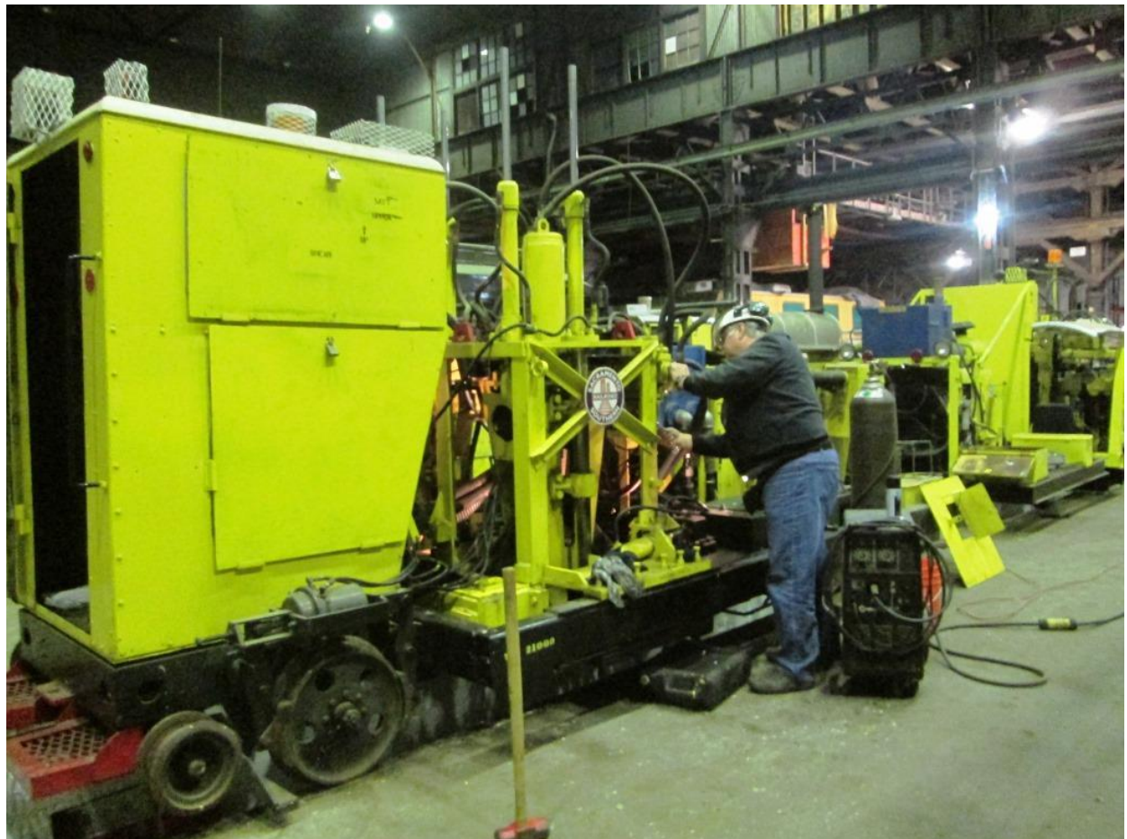
Chris C. working to cure the ailing tie-shear
